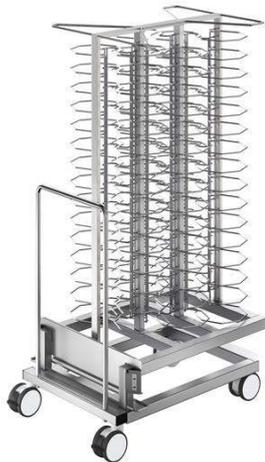
**922760 (TRBA92PL2021C)** Banquet trolley with rack holding 92 plates for 20 GN 2/1 oven and blast chiller freezer, 85mm pitch
